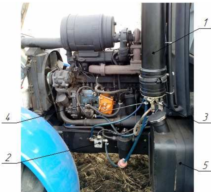
Fig. 1. The tested tractor with installed sensors: 1 - additional tank with the installed TKLS-L fuel level sensor; 2 - DFM-90A-P flow meter; 3 - three-way valve; 4 - high pressure fuel pump; 5 - regular fuel tank
