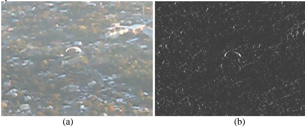
Fig. 1. (a) Image of a parachutist on the background of a locality in a mountainous area, (b) Brightness image of the difference between two frames
