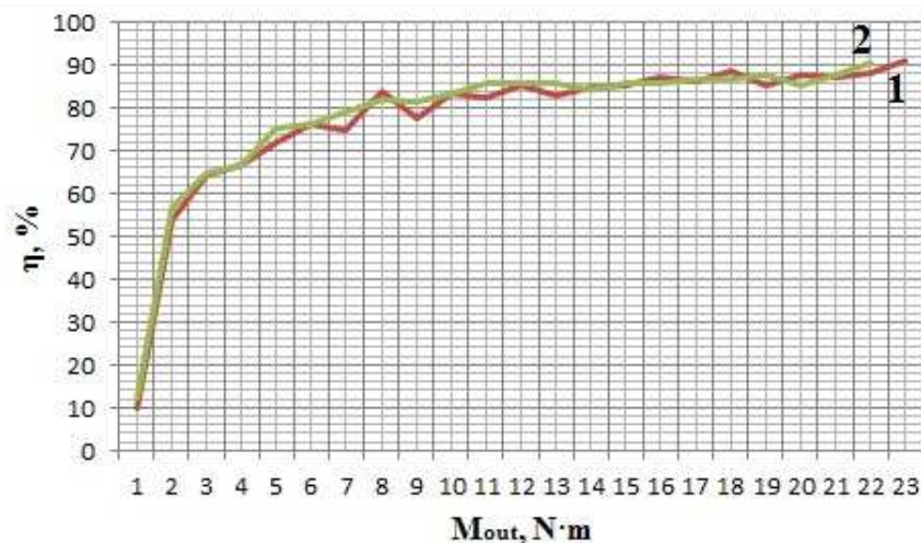
Fig. 11. Efficiency graph at 800 rpm: 1 – without magnetic field; 2 – with magnetic field
